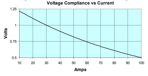
Compliance Voltage: 10 A Range 5.0 Vac rms maximum at 10 Amps
